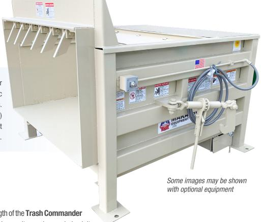
Use the Trash Commander<sup>™</sup> TANK<sup>®</sup> for weekly volumes of more than 100 cubic yards of uncompacted dry waste materials. Select a model based on the "feed (clear-top) opening" that will accommodate the largest items being processed in your application.
