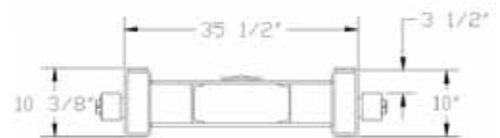
HOIST FRAME DETAIL
